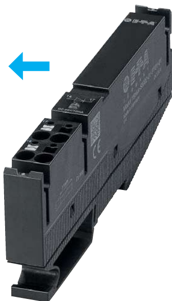
18plus-SM signalling module terminal 14 (aux. contact output) terminal 17 (GND for integral base load 10 mA with LED display)
